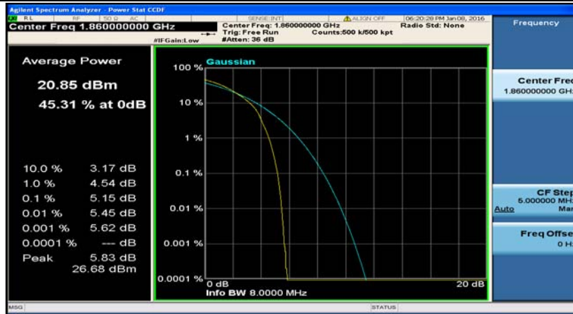
(Channel Bandwidth:20 MHz)_LCH_QPSK_50RB#25
