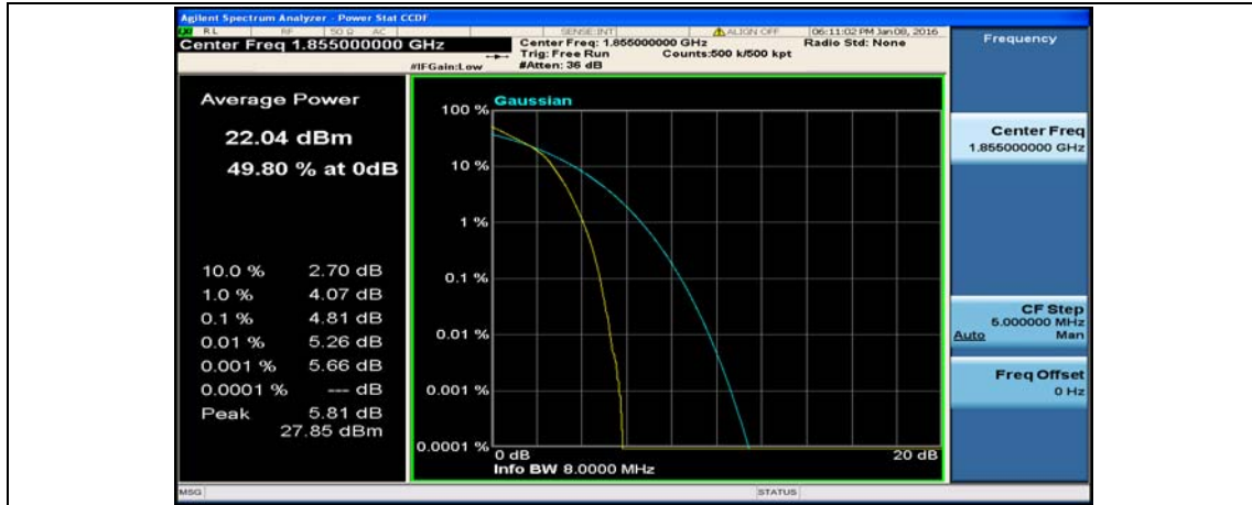
Channel Bandwidth: 10 MHz_MCH_16QAM_1RB#0
