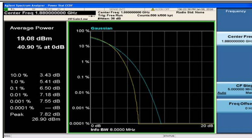
(Channel Bandwidth:20 MHz)_MCH_16QAM_50RB#25
