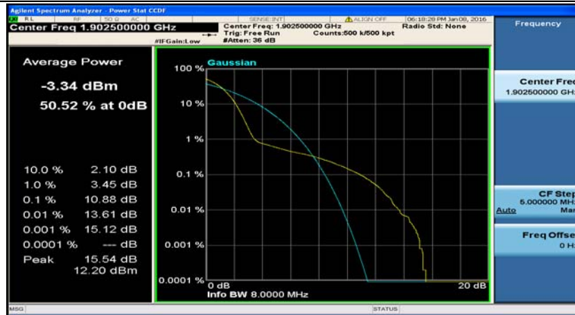
(Channel Bandwidth:15 MHz)_HCH_16QAM_37RB#0
