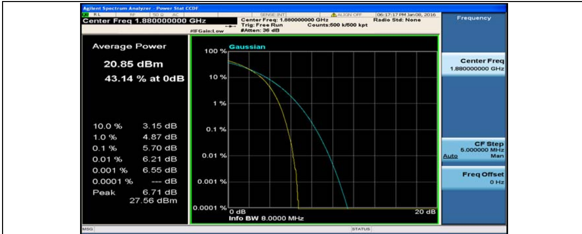
(Channel Bandwidth:15 MHz)_MCH_16QAM_75RB#0
