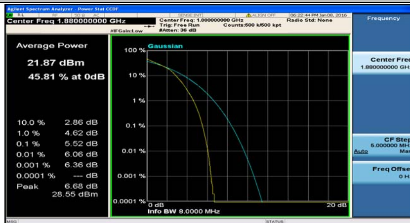
(Channel Bandwidth:20 MHz)_MCH_16QAM_50RB#50
