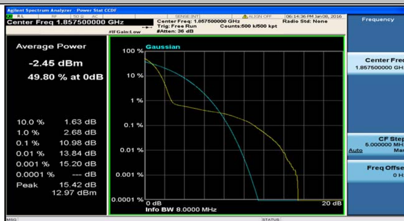
(Channel Bandwidth:15 MHz)_LCH_QPSK_37RB#0
