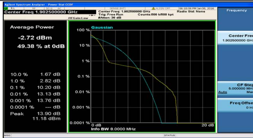
(Channel Bandwidth:15 MHz)_HCH_QPSK_37RB#0
