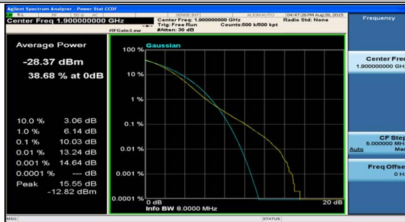
(Channel Bandwidth:20 MHz)_HCH_QPSK_50RB#0
