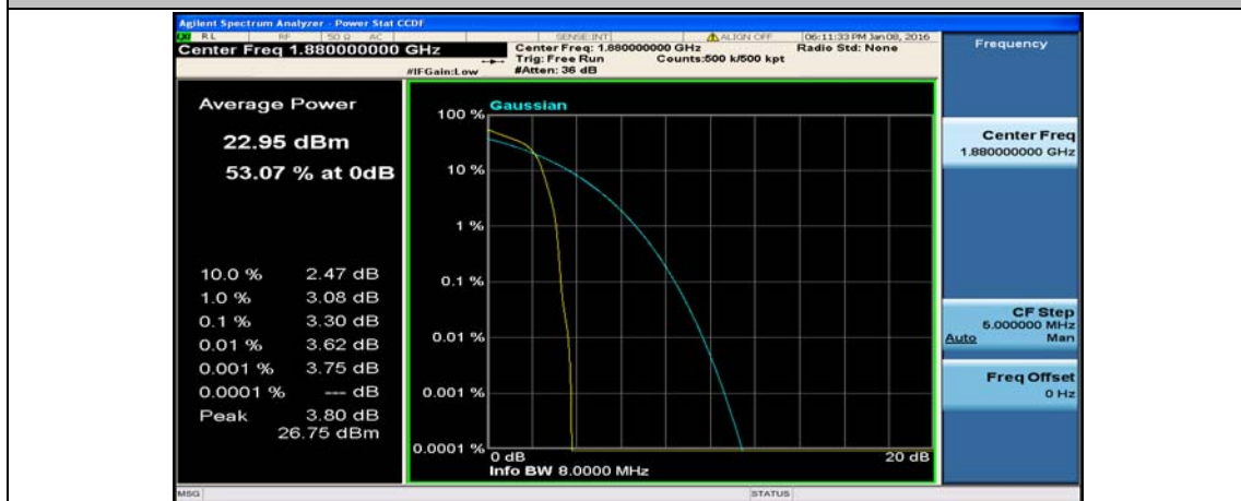
Channel Bandwidth: 10 MHz_MCH_16QAM_1RB#49
