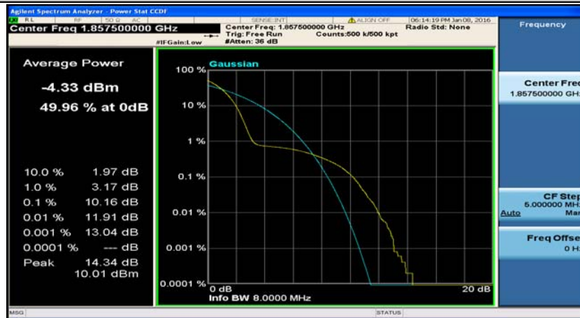
(Channel Bandwidth:15 MHz)_LCH_QPSK_1RB#37
