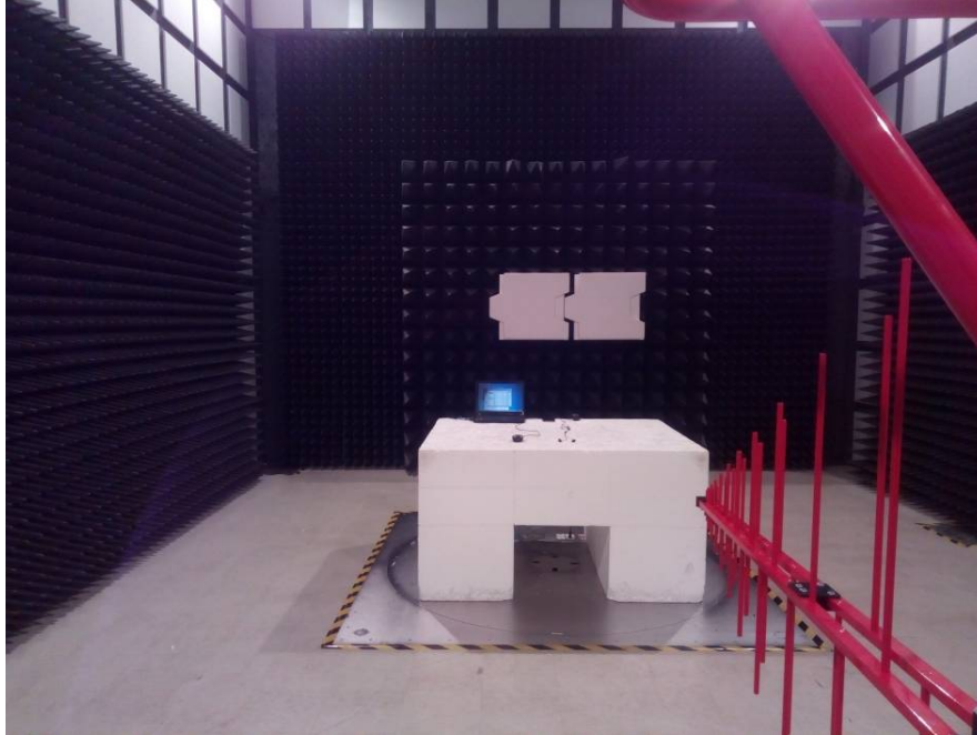
Radiated Emissions – Front View (Below 1 GHz)
