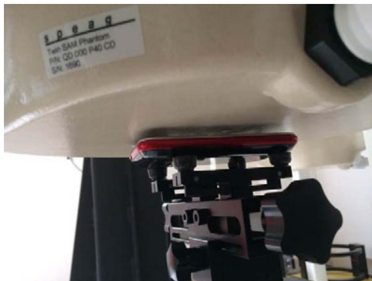
10mm Body-worn Front Side Setup Photo
