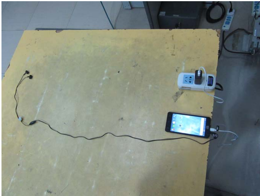
Conducted Emissions – Side View
