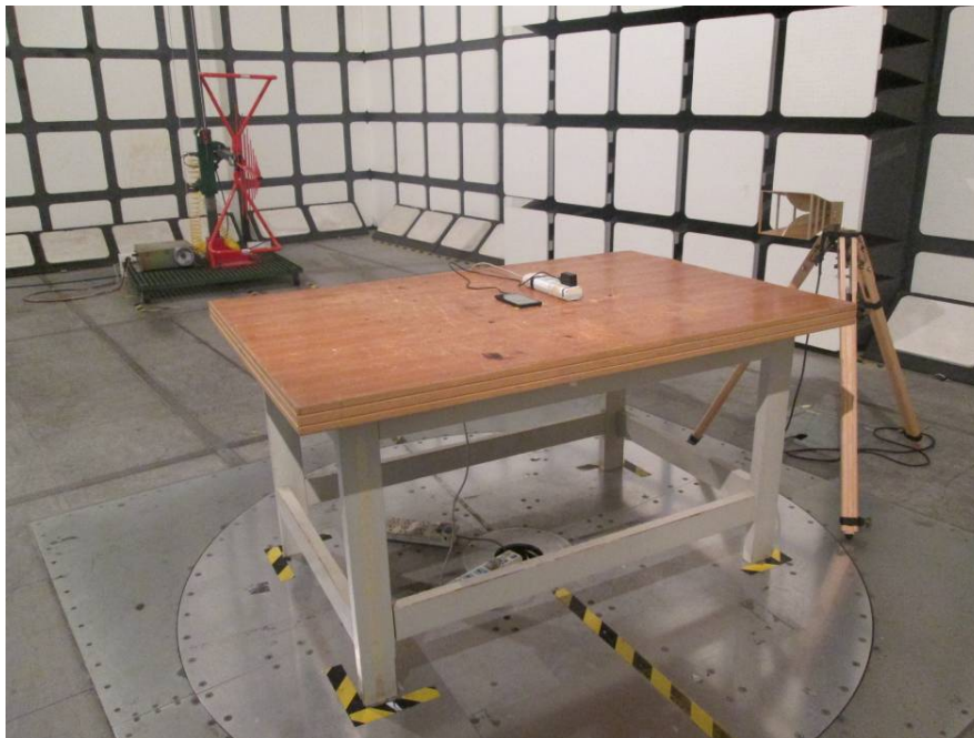
Radiated Emissions View (Below 1 GHz)
