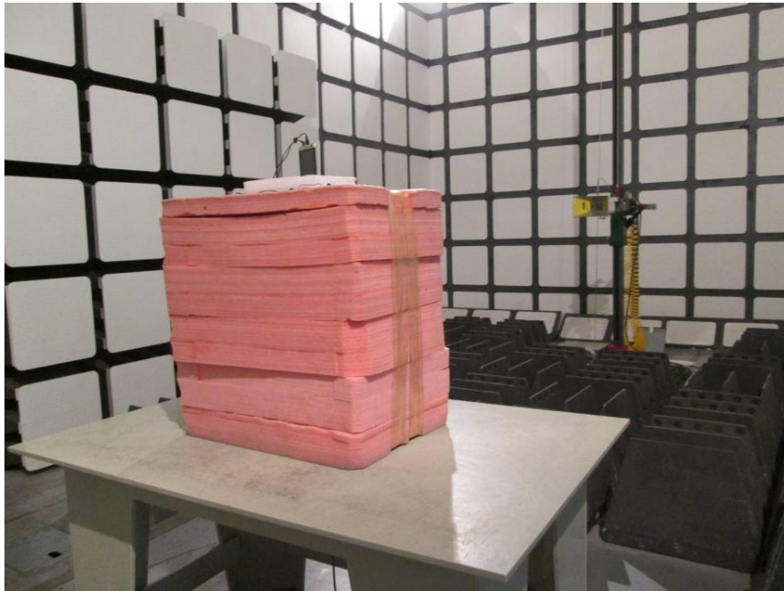
Radiated Emissions View (Above 1 GHz)
