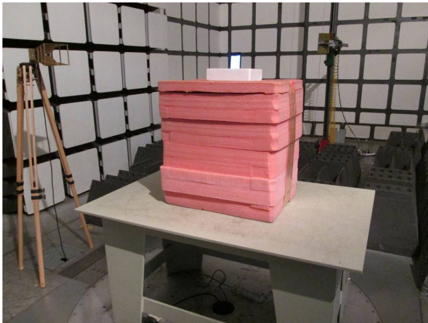
Radiated Emissions Test View (Above 1 GHz)
