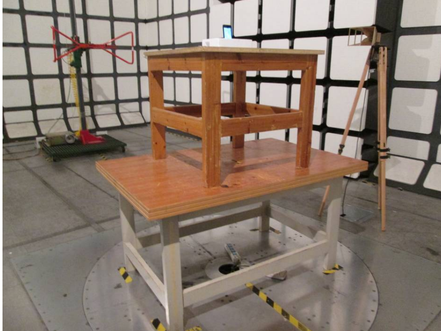
Radiated Emissions Test View (Below 1 GHz)
