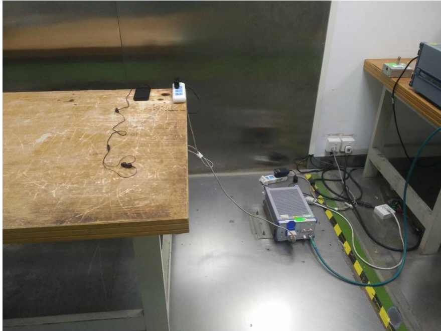
Conducted Emissions - Front View
