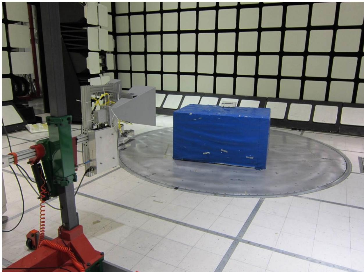
**Radiated Emissions – Antenna Vertical**
