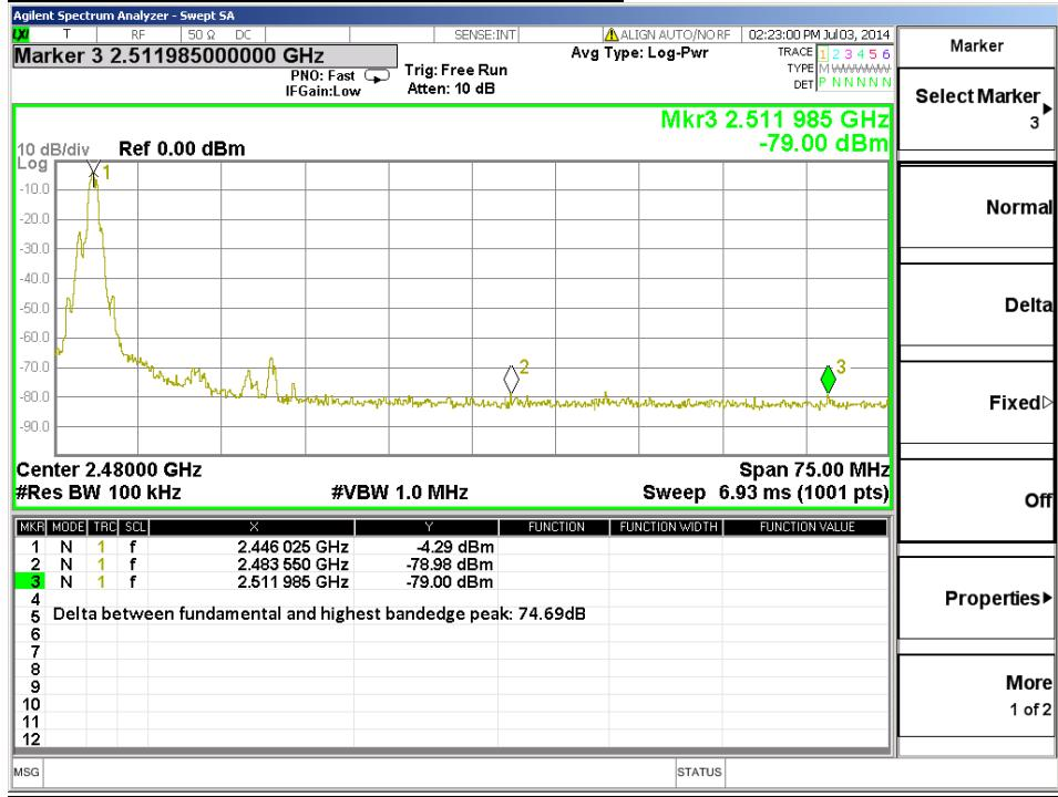
Calculated Worst Case Peak Level at Upper Band Edge based on above relative measurement and Maximum Peak Field Strength: Peak Level: (99.06dBuV/m - 74.69dB) = 24.37dBuV/m, Limit: 74dBuV/m, Margin: -49.63dB
