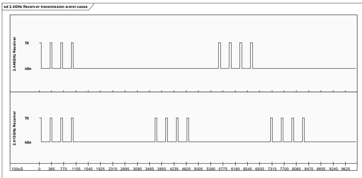
1. Receiver transmit at 2.415GHz. 4 pulses of about 65uS in a 3.63mS window. See attached file Receiverworstcase. (Error mode, ACK response to id message)
