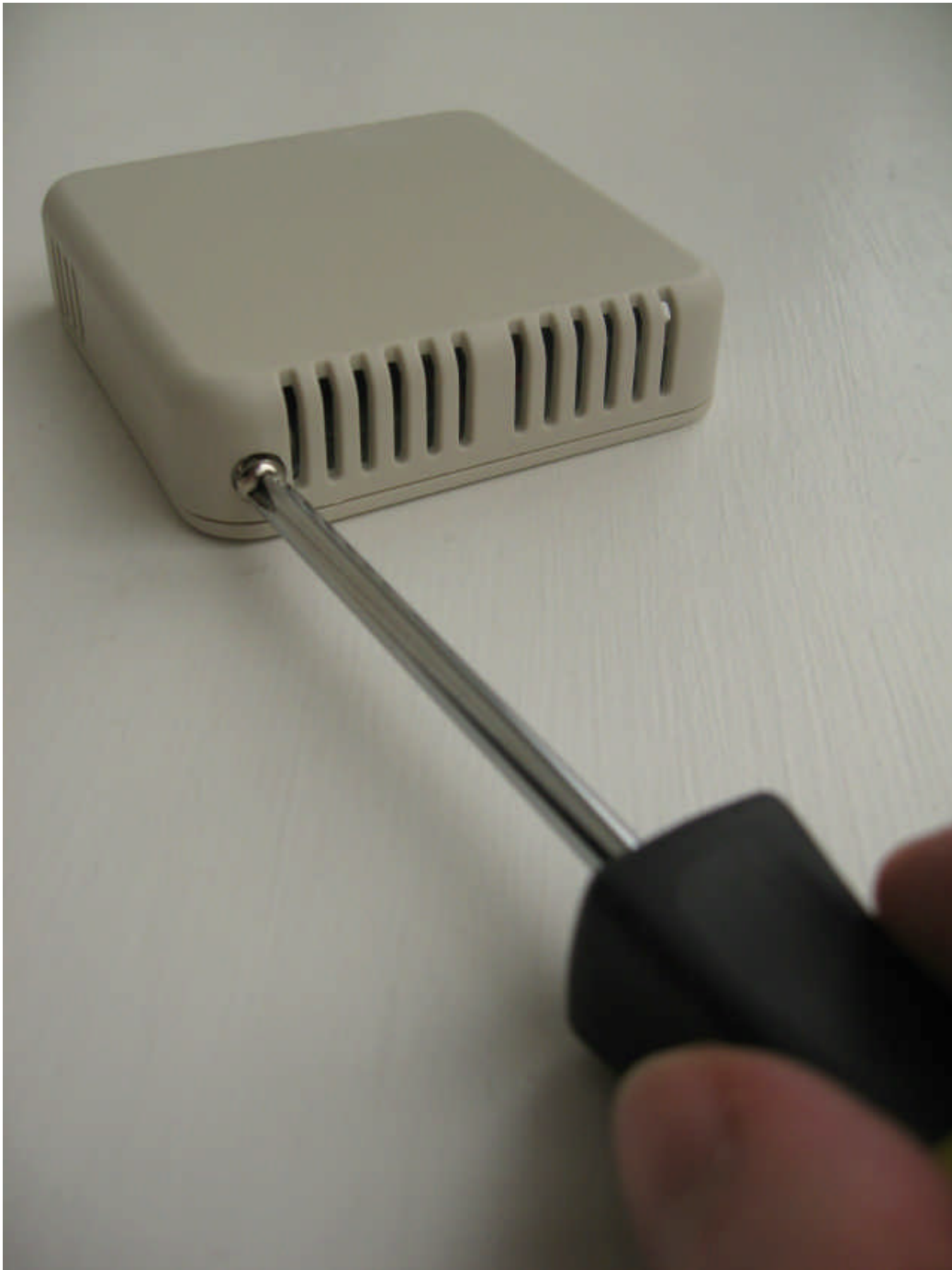
Fig. 1.0 WDC Tamper Screw Removal
