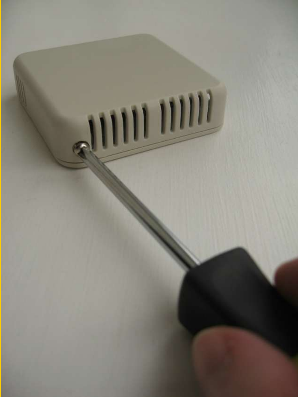
Fig. 1.0 WDC Tamper Screw Removal
