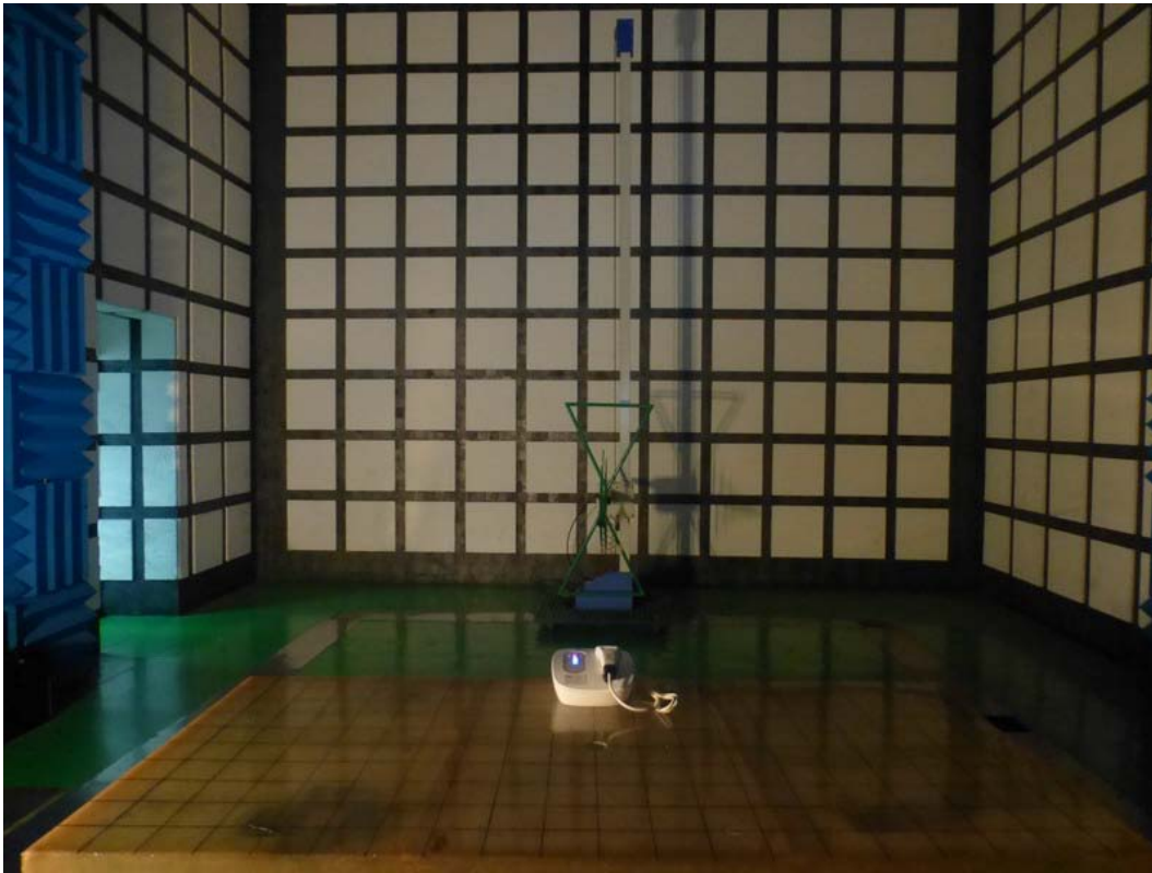
Photograph 4: Radiated Emission Test Configuration, (30-1000MHz) Back
