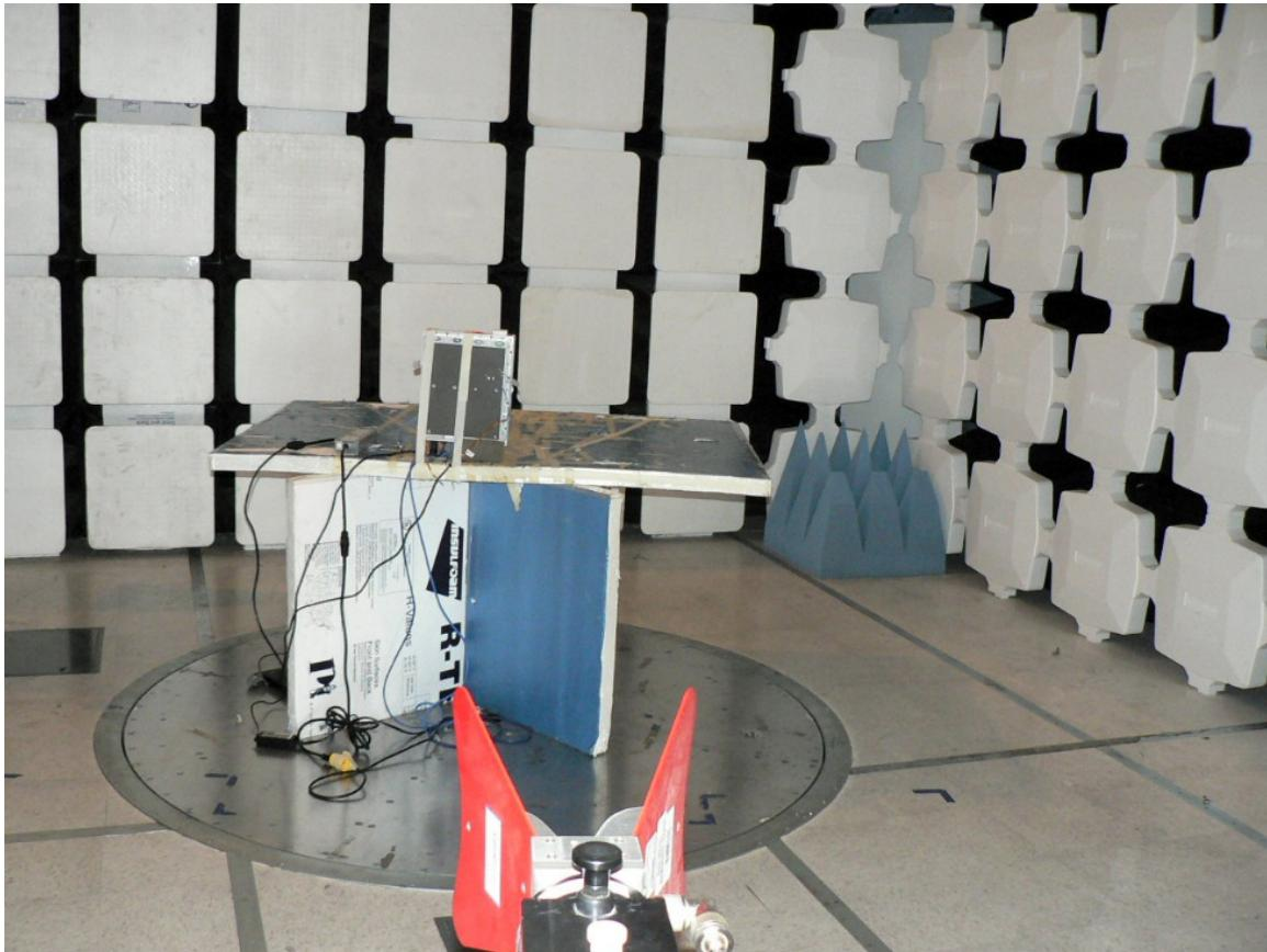
Radiated TX Spurious (1-18GHz back):
