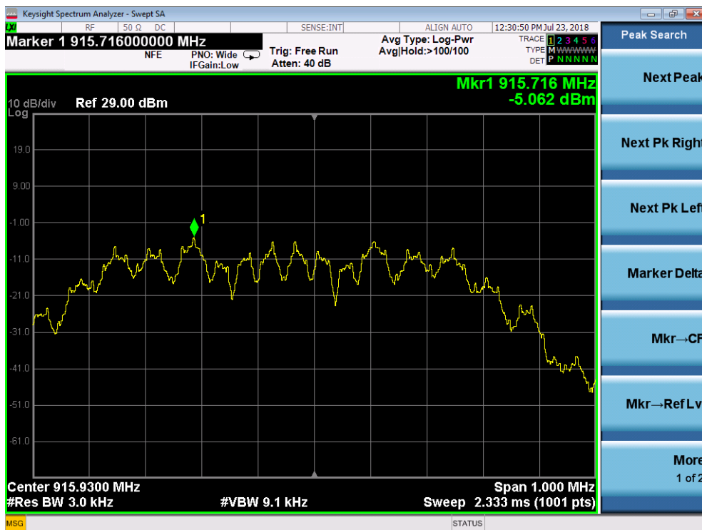
Figure 23-Peak Spectral Density.3kHz RBW 916MHz operation.
