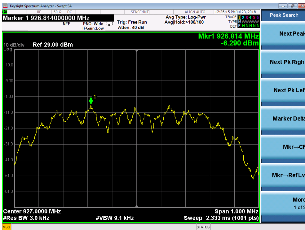
Figure 25-Peak Spectral Density.3kHz RBW 926MHz operation.
