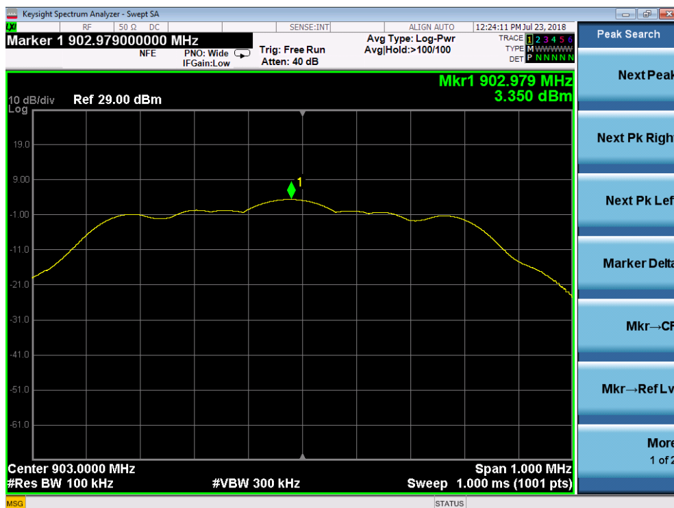
Figure 22-Peak Spectral Density.100kHz RBW 903MHz operation.
