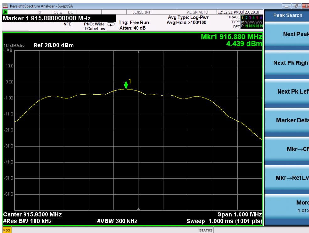
Figure 24-Peak Spectral Density.100kHz RBW 916MHz operation.
