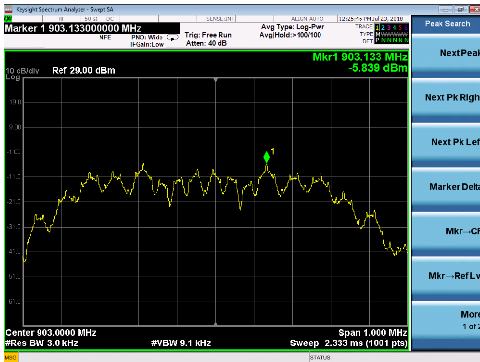
Figure 21-Peak Spectral Density.3kHz RBW 903MHz operation.
