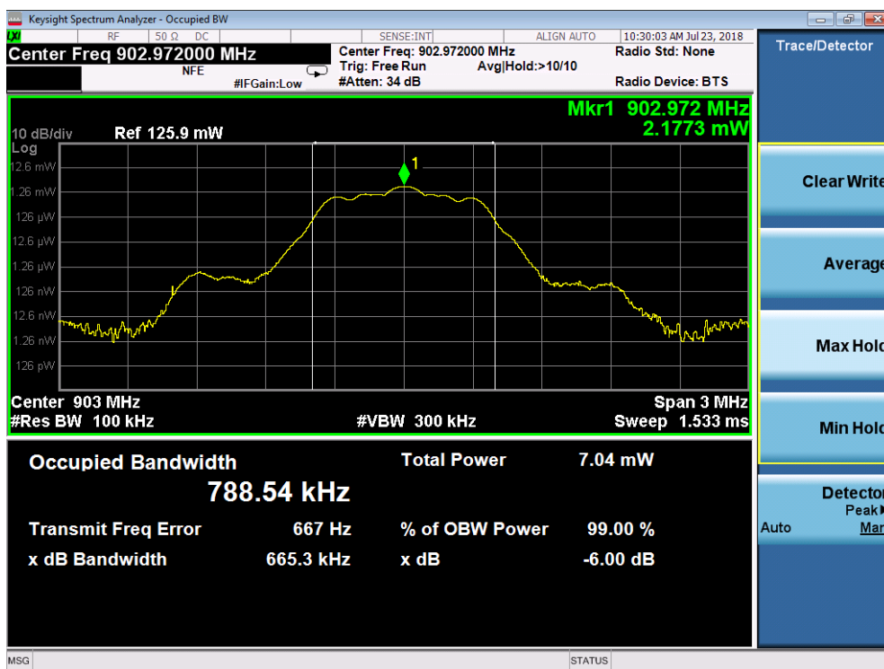
Figure 15 Bandwidth at 6dB Point. 903MHz Operation
