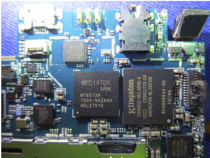
EUT –Main Chip View
