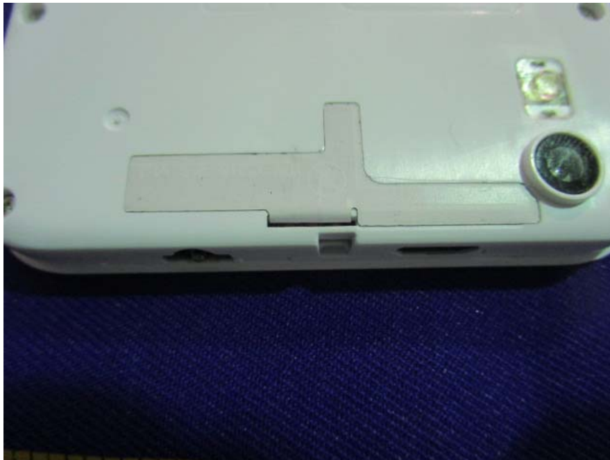
EUT –BT&WiFi Antenna View
