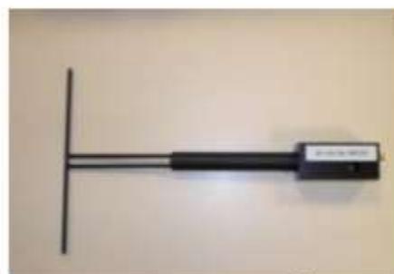
Figure 1 – Satimo COMOSAR Validation Dipole
