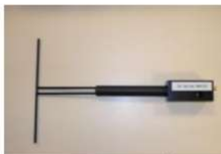
Figure 1 – Satimo COMOSAR Validation Dipole
