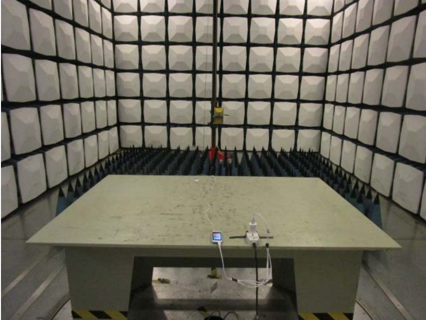
Radiated Emission - Rear View (Above 1GHz)
