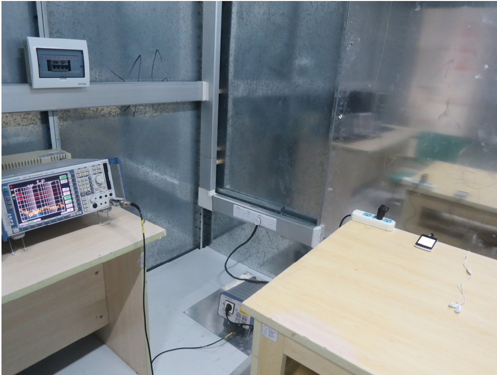
FCC RADIATED EMISSION TEST SETUP
