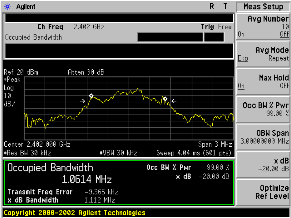
TEST PLOT OF BANDWIDTH FOR LOW CHANNEL
