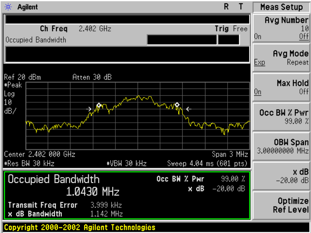
TEST PLOT OF BANDWIDTH FOR LOW CHANNEL
