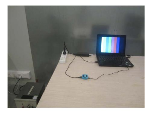
Radiation Emission Test Setup (30MHz to 1GHz)
