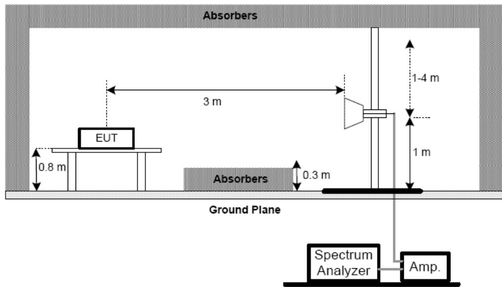
(C) For radiated emissions below 30MHz
