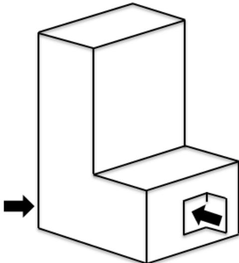
There are two power switches, one is on the back and the other is inside of the service door. Both of them need to be ON to operate the game.
