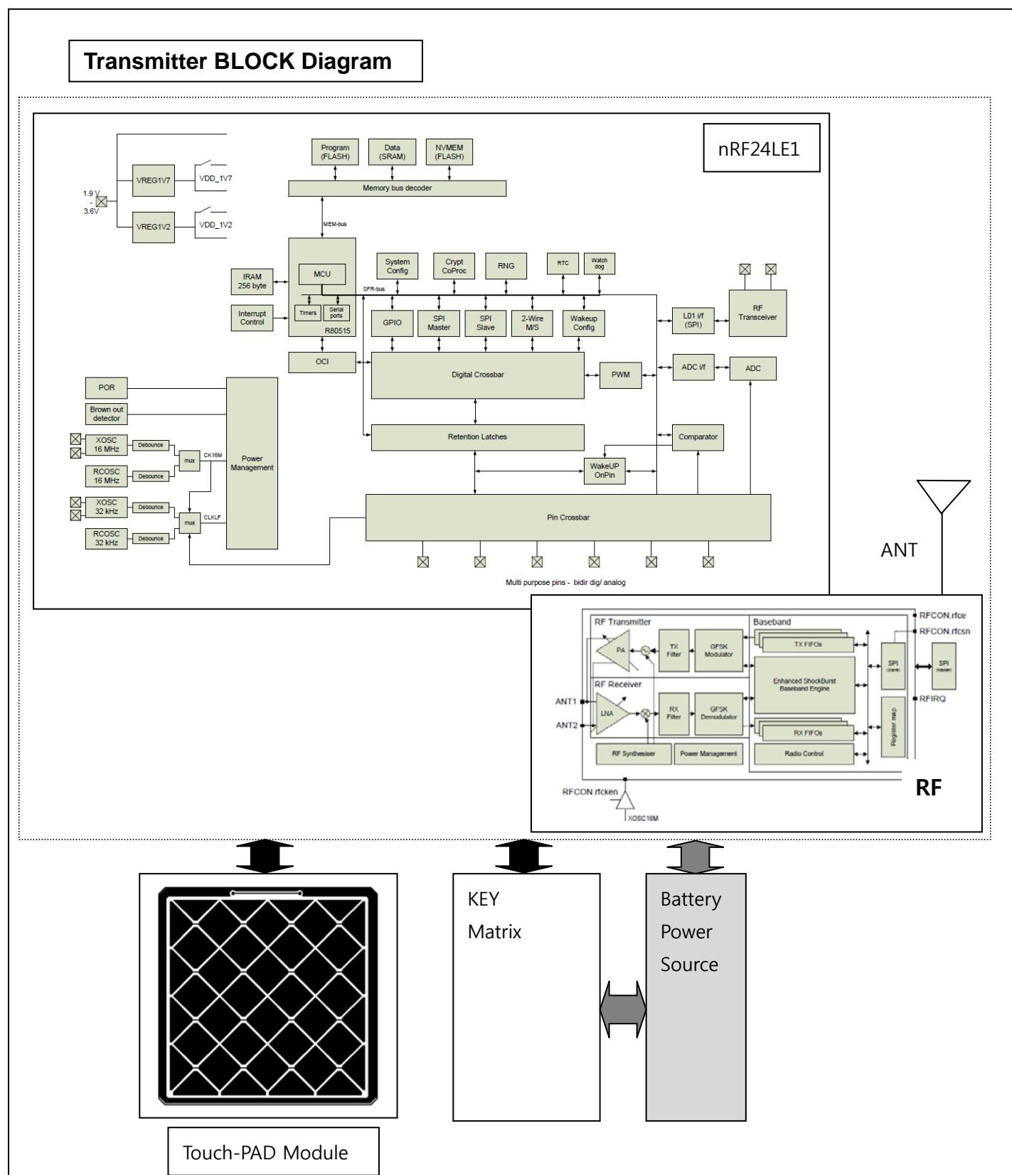
Touch Air (ITV-R01) Remote Controller has configured Touch PAD Module, Key Function and nRF24LE1
