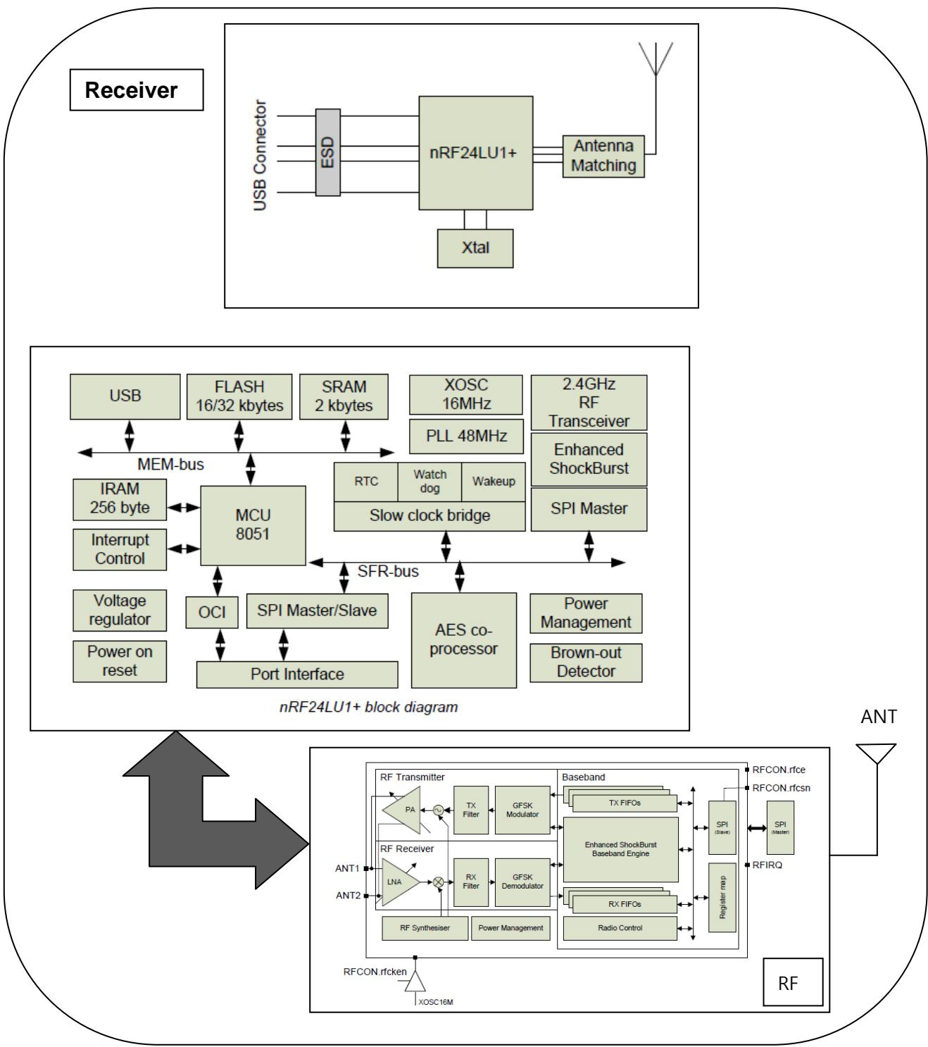
The nRF24LU1+ is a unique single chip solution enabling ultra compact USB dongles for wireless peripherals. The USB Dongle supports Full speed 2.0 compliant device controller
