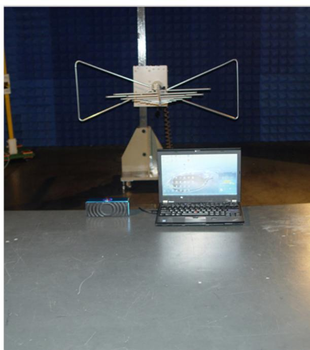
**Radiated emissions test > 1GHz**
