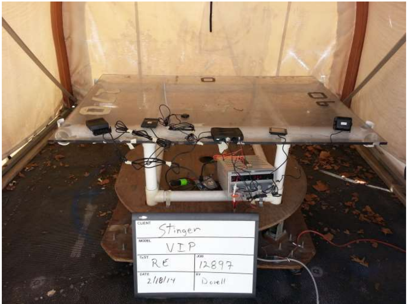
Photograph 2: Radiated Emission Test Configuration, Back
