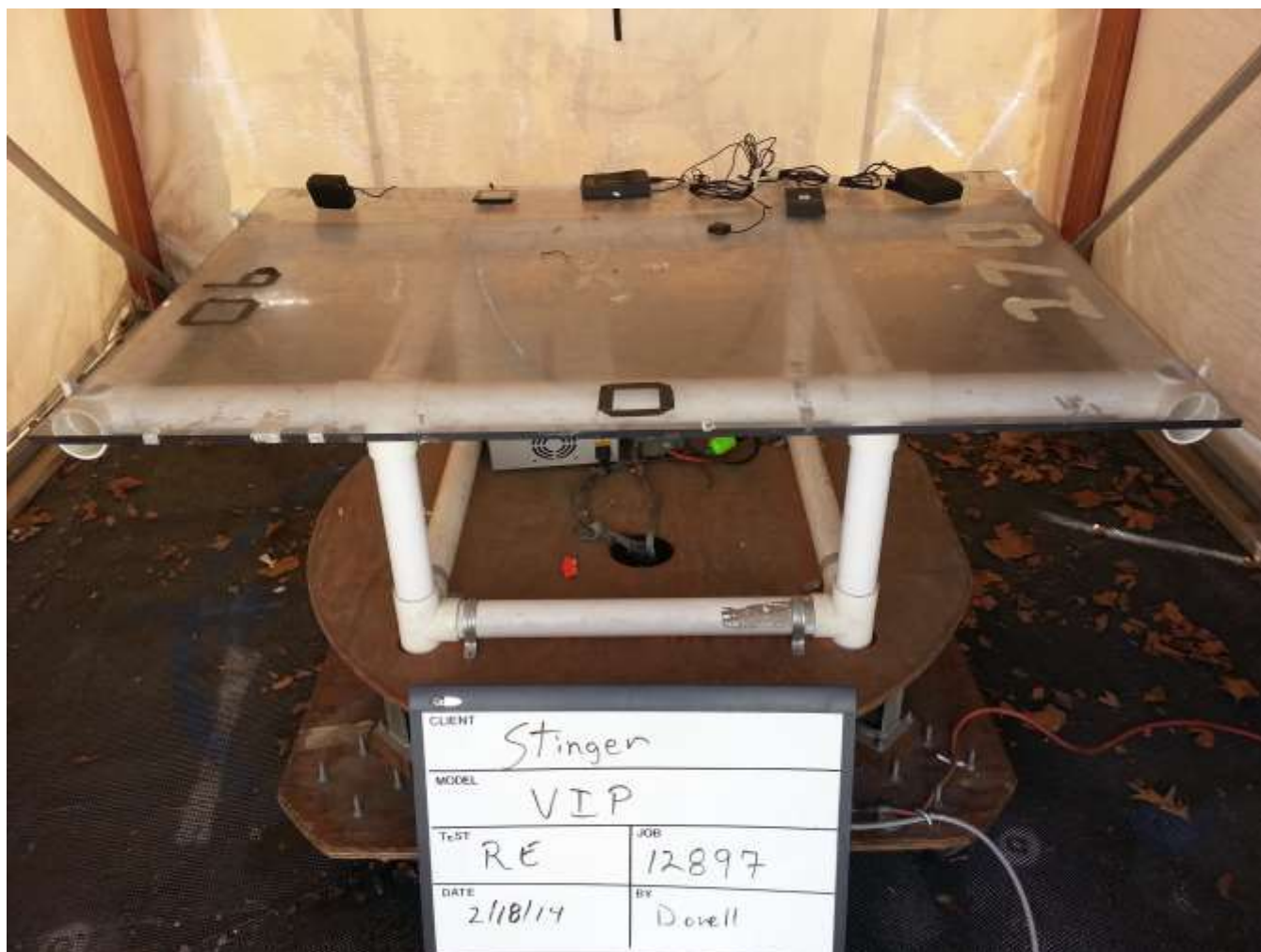
Photograph 1: Radiated Emission Test Configuration, Front
