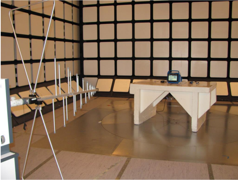
Photograph 1. Radiated spurious emission test.
