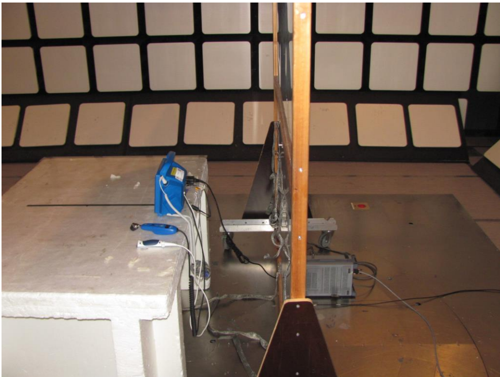
Photograph 2. Conducted emissions at mains ports emission test.
