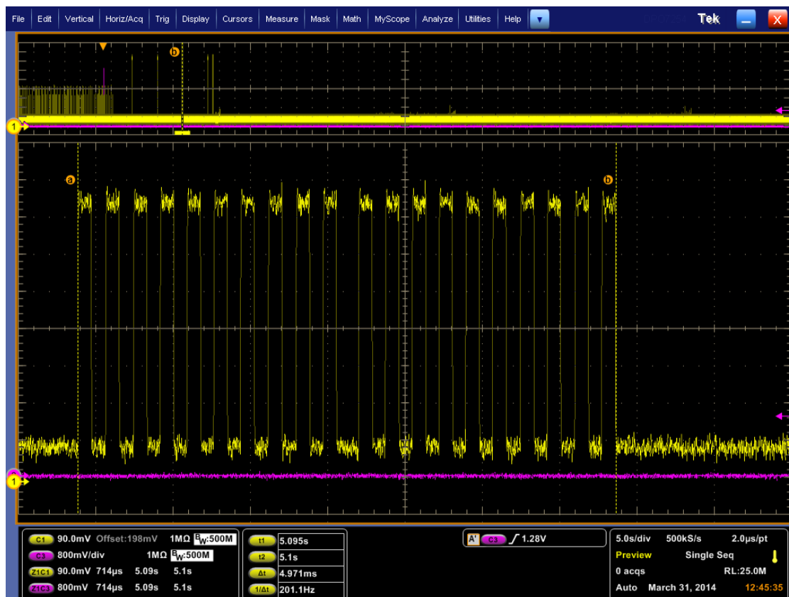
Figure 5: 5280MHz, client transmissions after 200ms: (20 \times 0.14\text{ms}) \times 4 + 10 \times 0.07\text{ms} = 11.2 + 0.7 = 11.9\text{ms} . (radar pulse purple curve, EUT highest on yellow curve).
