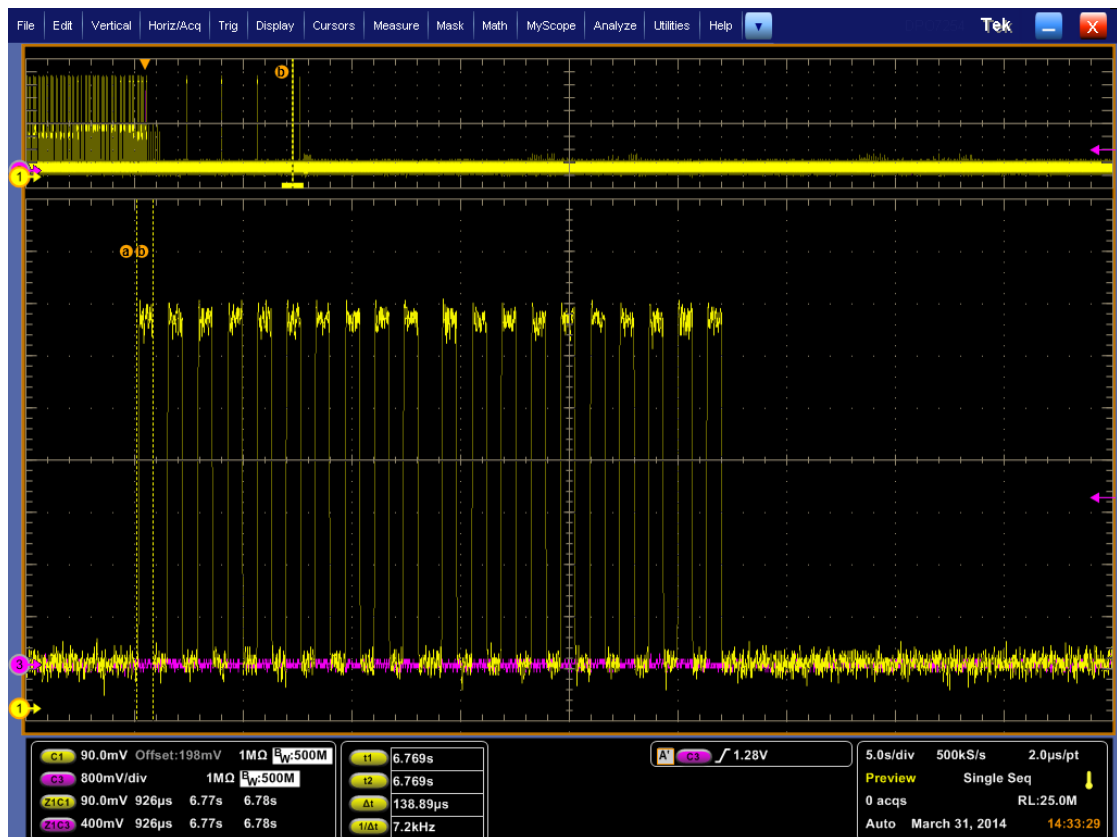
Figure 11: 5580MHz, client transmissions after 200ms: (20 \times 0.14 \text{ ms}) \times 4 + 10 \times 0.07 \text{ ms} = 11.2 + 0.7 = 11.9 \text{ ms}
