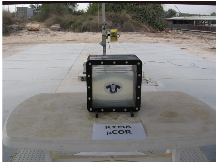
Figure 2. Radiated Emission Test Setup
