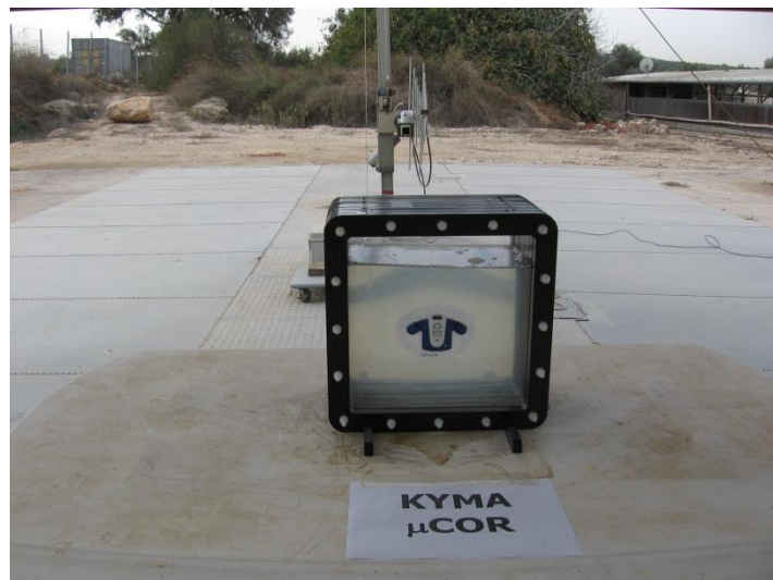
Figure 3. Radiated Emission Test Setup
