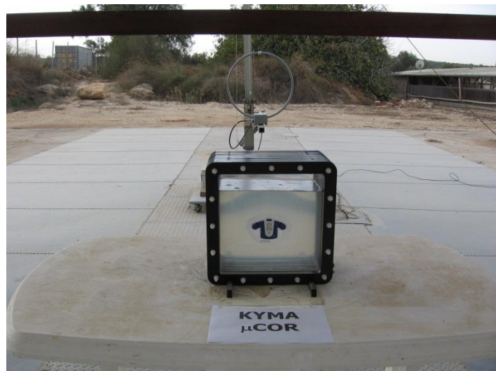
Figure 5. Radiated Emission Test Setup
