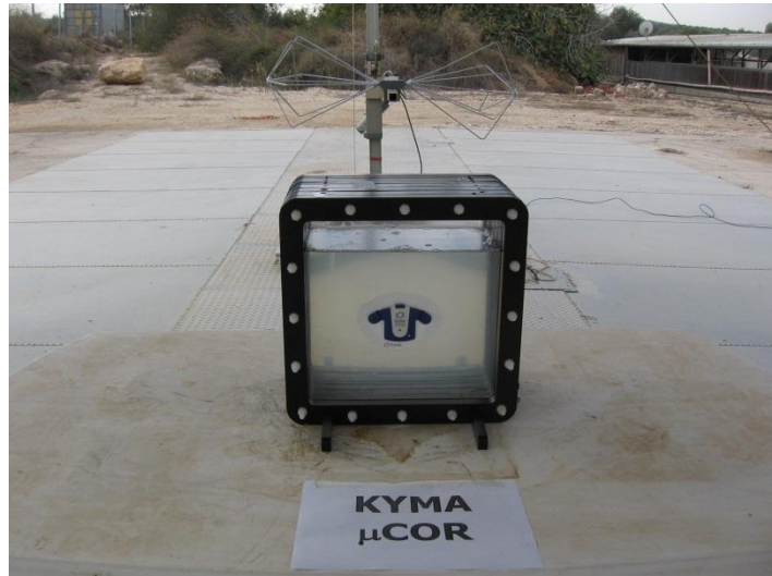
Figure 4. Radiated Emission Test Setup
