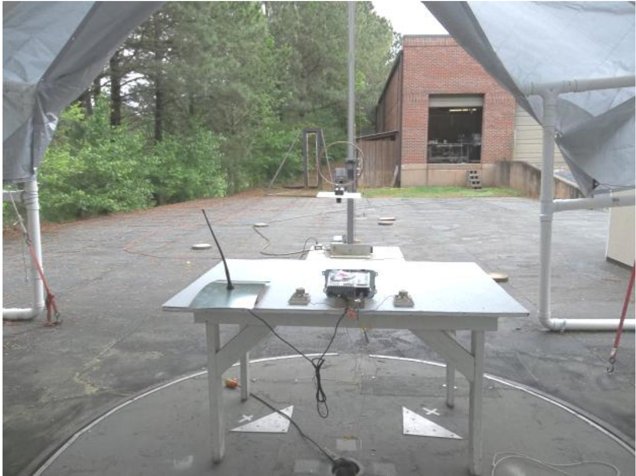
Figure 5. Radiated Emissions Test Setup (9 KHz to 30 Mhz)
