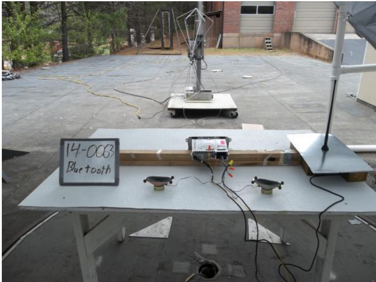
Figure 2. Radiated Emissions Test Setup (30-200 MHz)
