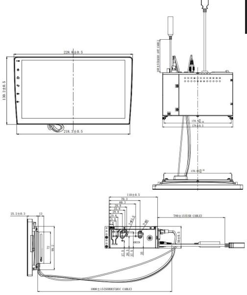
FX575 Dimensions: FX575 Weight: 2Kg (Including Accessary)
