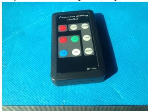
II: The products can be controlled by the wireless remote in high frequency(433MHZ).The remote is easily operated in 20meters when it is point to the battery box.
