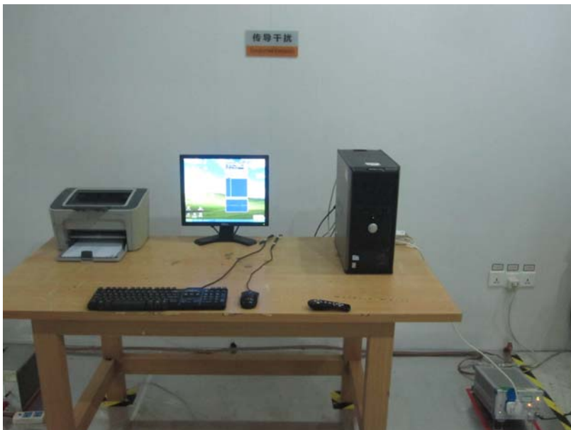
Photo of Setup for Conducted Emission
