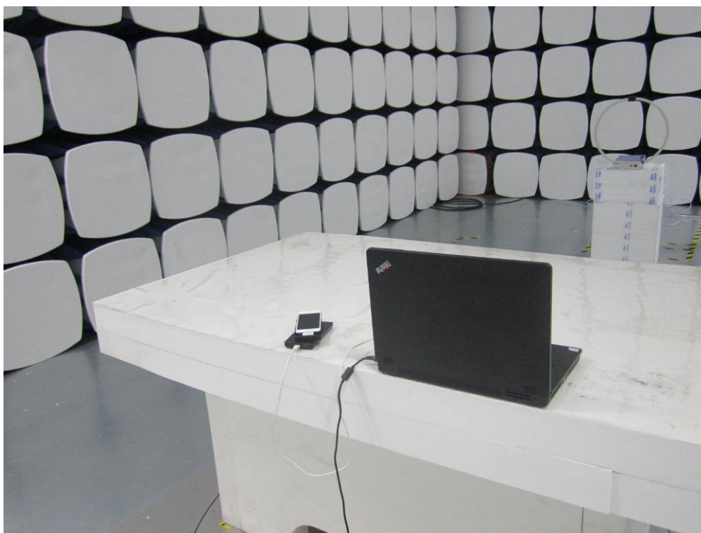
Radiated Spurious Emissions Test Setup Below 30 MHz - Front View
