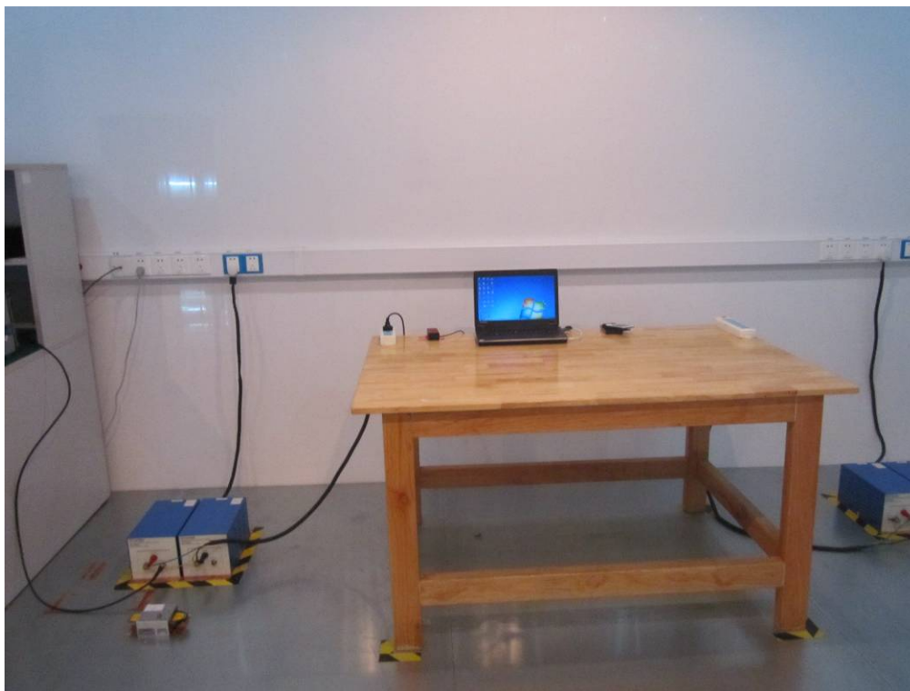
Conducted Emissions Test Setup Front View
