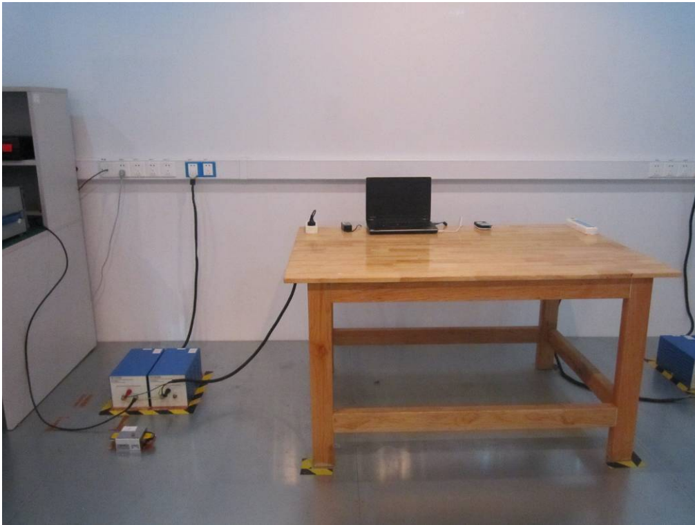
Conducted Emissions Test Setup Front View
