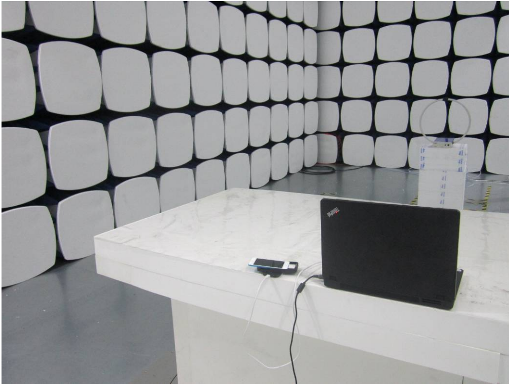
Radiated Spurious Emissions Test Setup Below 30 MHz - Front View
