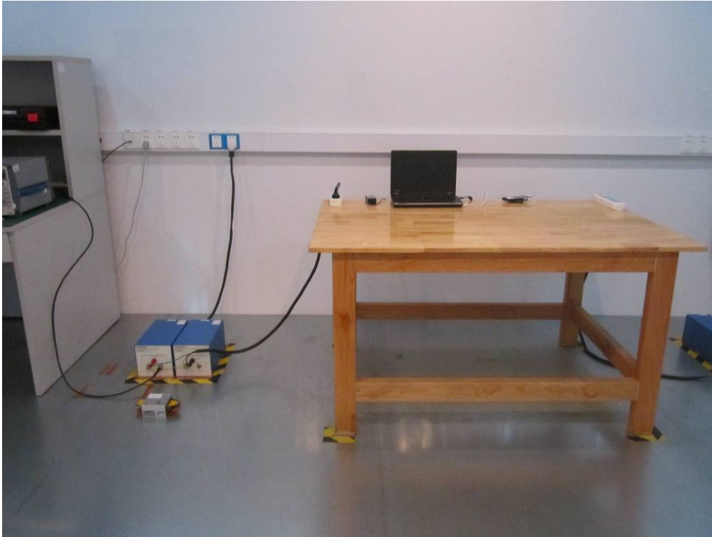
Conducted Emissions Test Setup Front View
