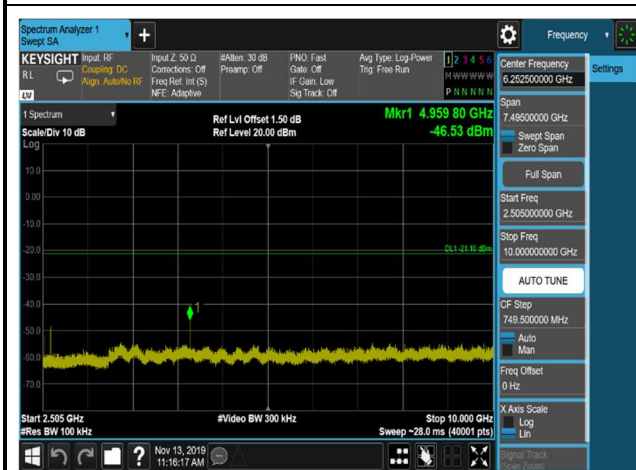
DQPSK,2402MHz,2DH5,Plot 1,Band Edge
