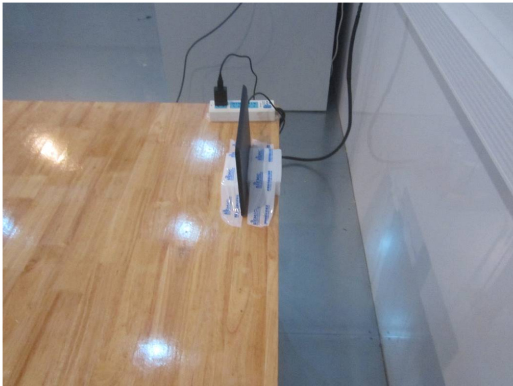
Conducted Emissions Test Setup Side View
