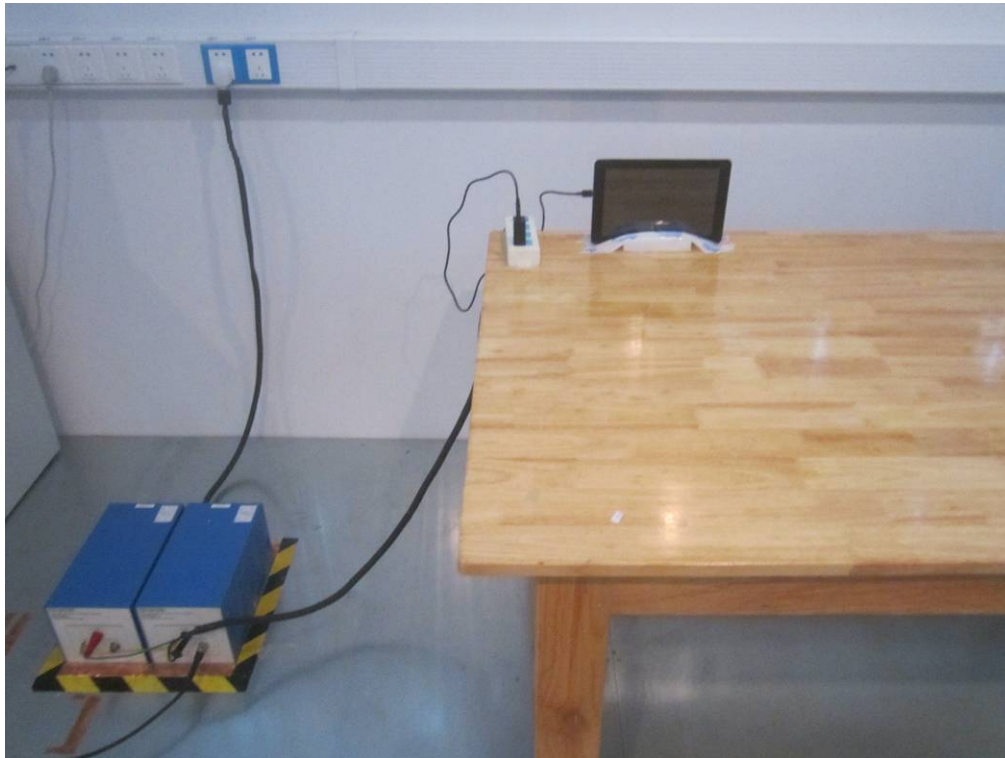
Conducted Emissions Test Setup Front View
