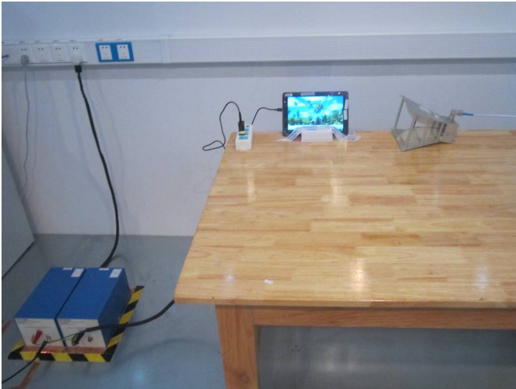
Conducted Emissions Test Setup Front View
