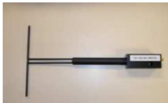
Figure 1 – Satimo COMOSAR Validation Dipole
