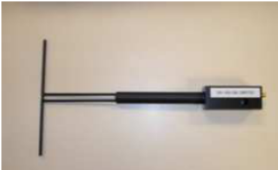
Figure 1 – Satimo COMOSAR Validation Dipole
