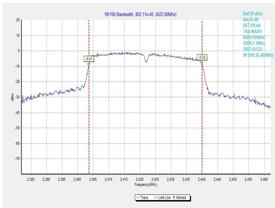
Fig.A.8.10 99% Occupied Bandwidth: (802.11n-HT40, Ch 3)
