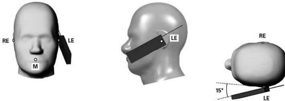
Fig 9.4 Illustration for Tilted Position
