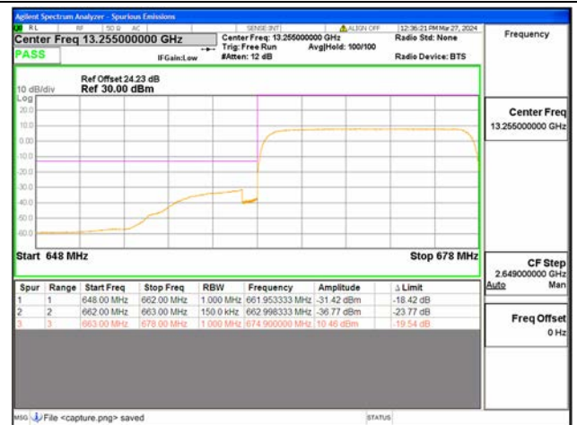
B71 / 15MHz / Low CH / QPSK / FULL RB
