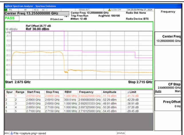
B41 / 15MHz / High CH / QPSK / FULL RB
