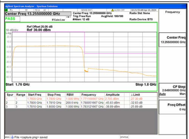
B66 / 20MHz / High CH / QPSK / FULL RB
