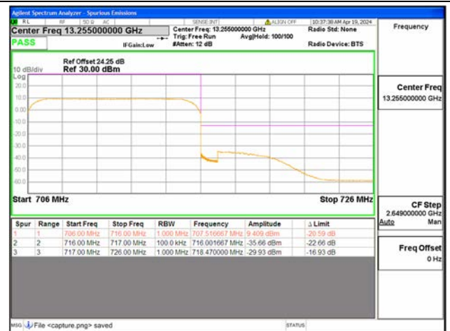
B12 / 10MHz / High CH / QPSK / FULL RB
