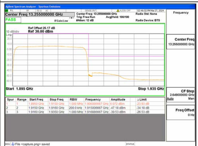
B25 / 20MHz / High CH / QPSK / FULL RB
