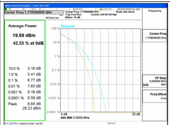
B66 / 3MHz / High CH / 64QAM
