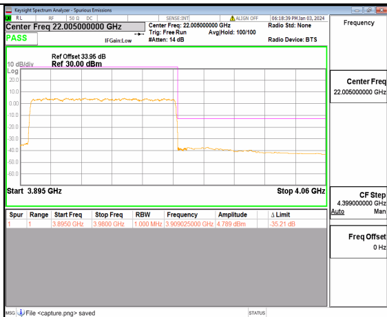
n77(3700-3980MHz) 80M DFT-s-OFDM QPSK Outer_Full High
