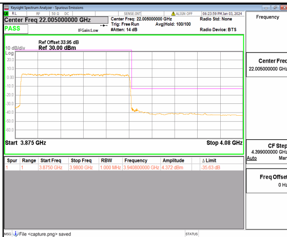
n77(3700-3980MHz) 100M DFT-s-OFDM BPSK Outer_Full High
