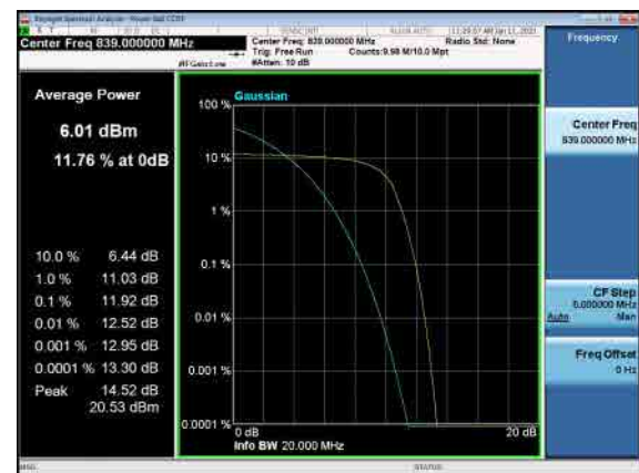
B66_N5(20M)_DFT-s-OFDM_QPSK_ High CH
