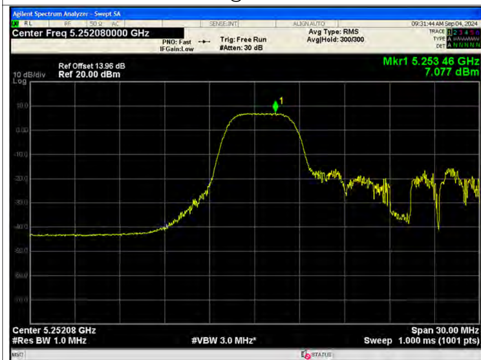
PSD NVNT ax20 52@37 5260MHz Ant1 SISO
