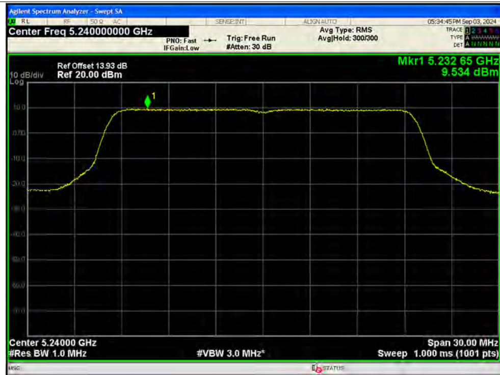
PSD NVNT be20 5260MHz Ant2 SISO
