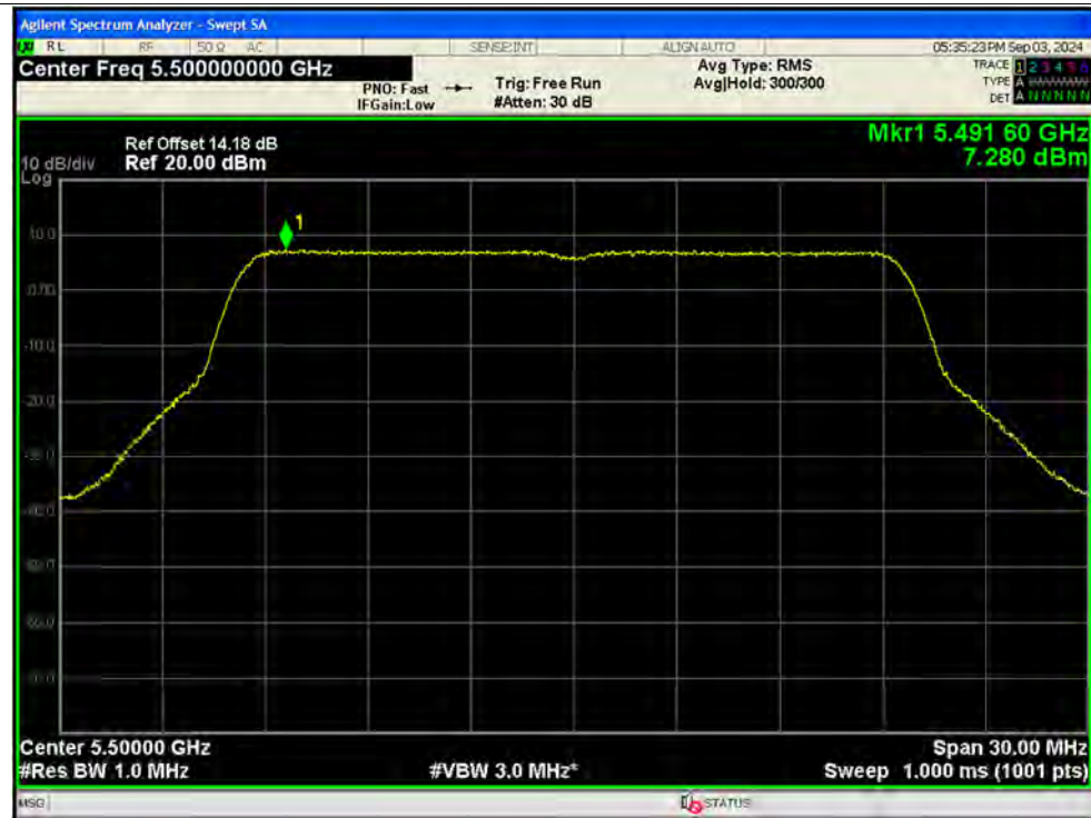
PSD NVNT be20 5600MHz Ant2 SISO
