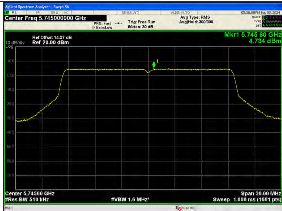
PSD NVNT be20 5745MHz Ant2 SISO
