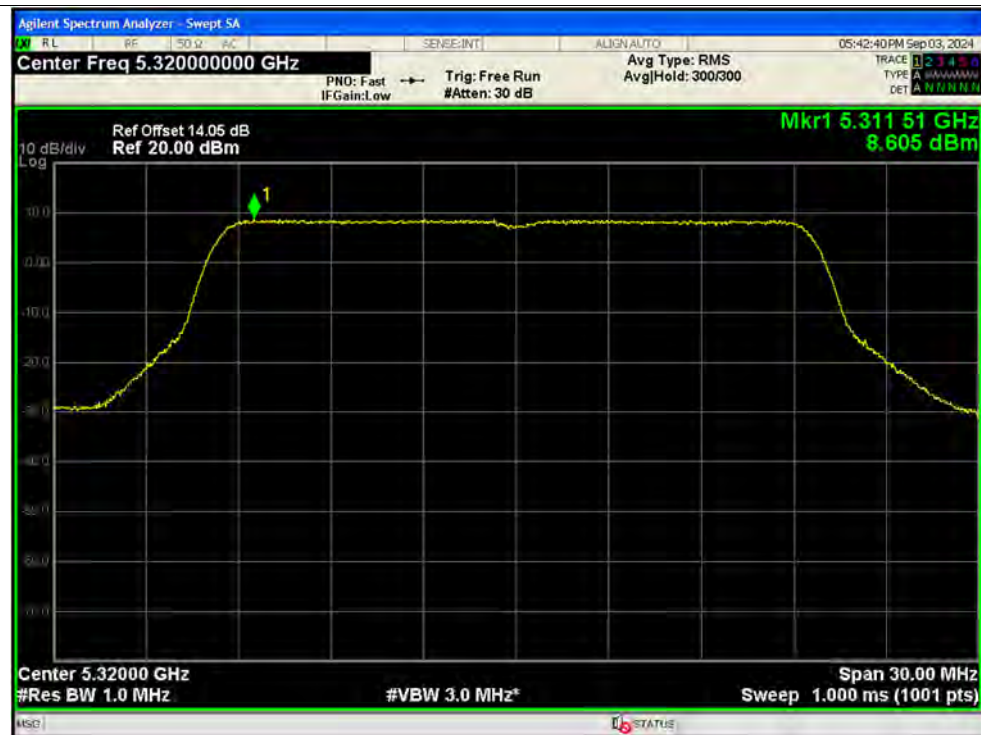
PSD NVNT be20 5320MHz Ant2 SISO
