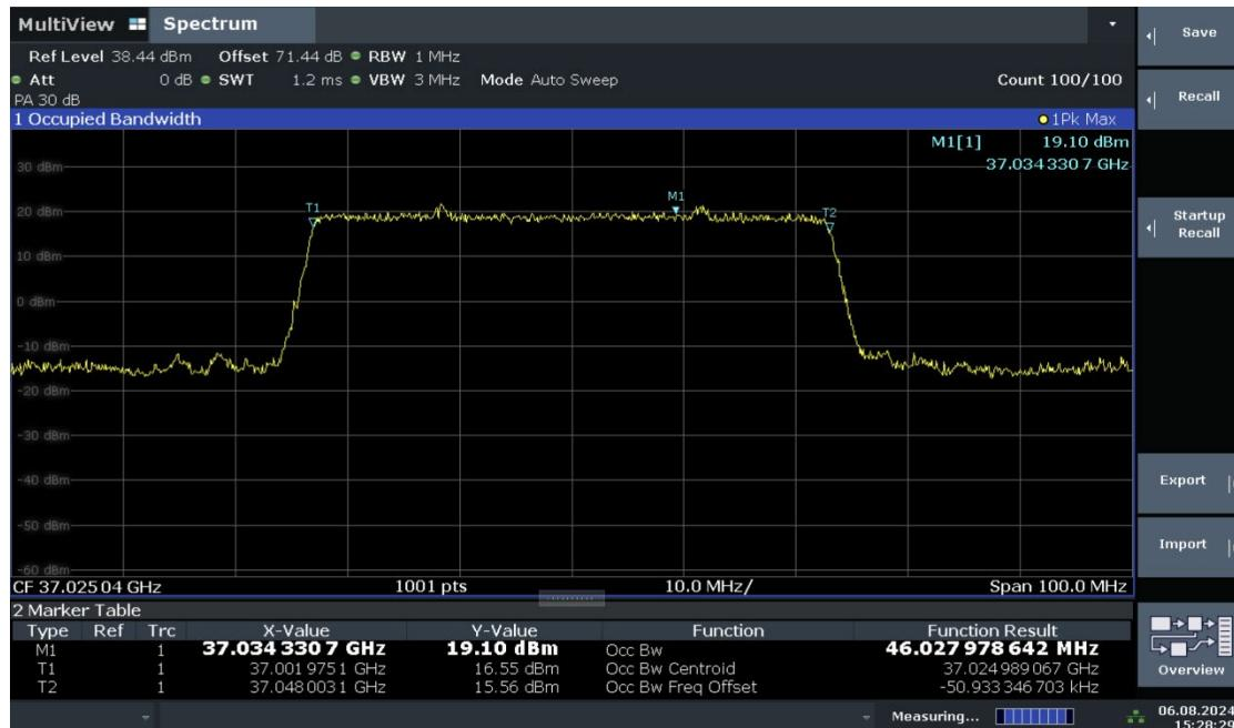
**n260, Module 0, 50MHz, LOW CH, PUSCH DFT QPSK (99% BW)**
