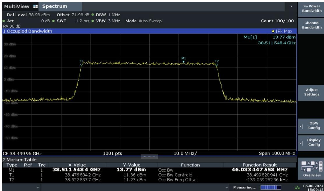
n260, Module 0, 50MHz, MID CH, CP-OFDM QPSK (99% BW)
