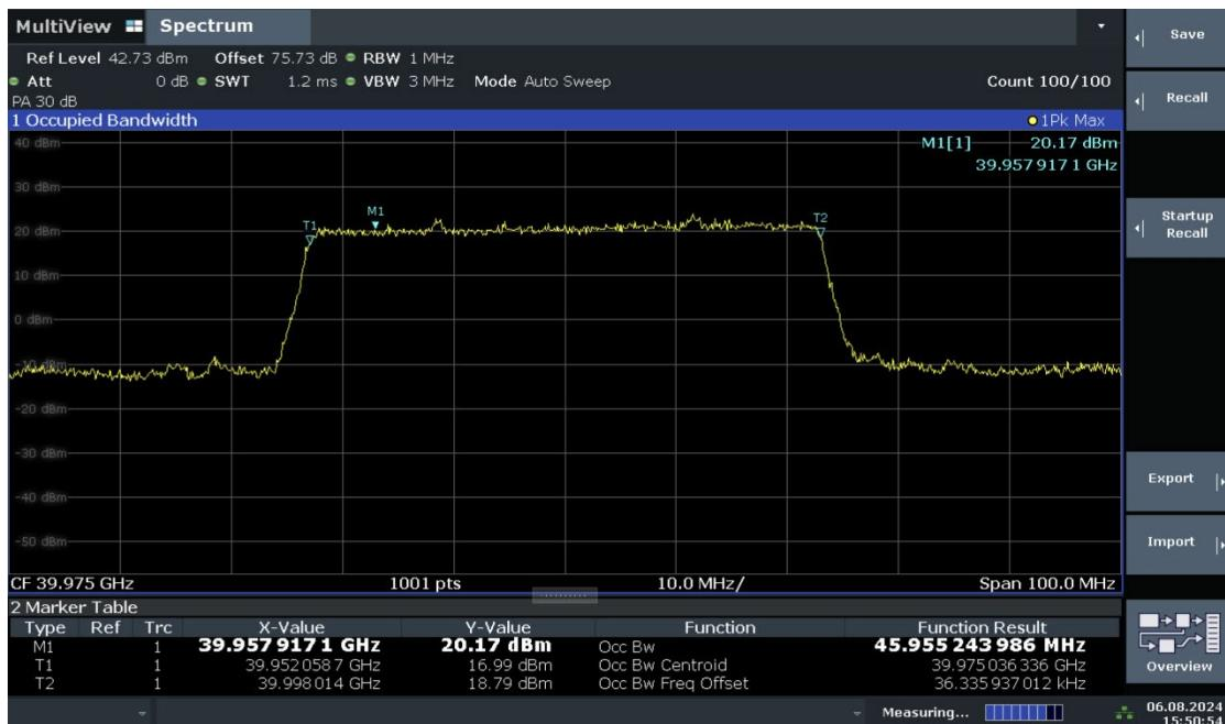
**n260, Module 0, 50MHz, HIGH CH, PUSCH DFT QPSK (99% BW)**
