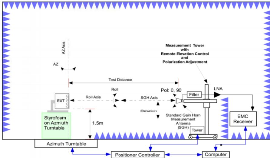
(For the test frequency from 40GHz to 220GHz)
